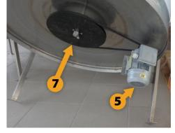
Check the V-pulley at the bottom of the unit to ensure the secure fastening on the central shaft. Adjust it using the screw on the V-pulley if necessary. Check V-pulleys to ensure that they are in line and the V-belt is not twisted, also check the V-belt for tightness. If the V-belt is not on the pulley then place it.
