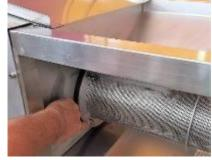
recommended to start the pressing always at a low speed, and to gradually increase the speed.
