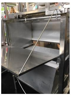
The knife (4) and the setup of the uncapping machine are arranged by the factory to fit the size of the ordered frame. For follow-up adjustments, place a frame into the frame stand. Set the exact fitting with the help of the clamps (2).
