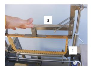
Press the treadle again and remove the uncapped frame from the clamps at the same time, place it on the uncapped frame receiver and restart the process.
