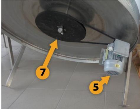
Check the V-pulley at the bottom of the unit to ensure the secure fastening on the central shaft. Adjust it using the screw on the V-pulley if necessary. Check V-pulleys to ensure that they are in line and the V-belt is not twisted, also check the V-belt for tightness. If the V-belt is not on the pulley then place it.
